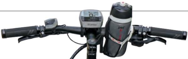
**Retrofit kit for the fixation of bottle cages** on Ahead stems by replacing the headset's top cap. Fits all regular bottle cages.
